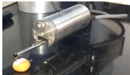
(Fig-4 Testing of specimen by surface profiler)
