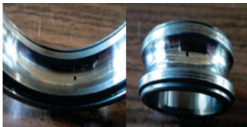
Figure 3: Artificial defects on the bearing components
