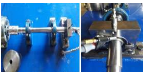
Figure 5: (a) Test rig (b) housing bearing.
