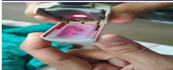
Figure2. Smudging of the light detecting photodiode of the probe with blue ink
