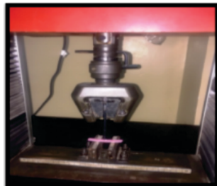
Fig 5: Transverse strength testing on UTM
