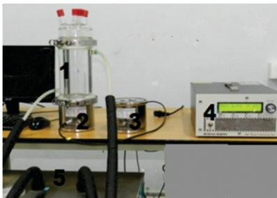
Fig.2. Sonoreaction assembly, 1: Glass reactor, 2, 3: Variable frequency generators, 4: Power supply unit, 5: Thermostat
