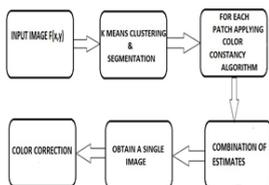
**Fig 3. Block diagram of proposed method**
