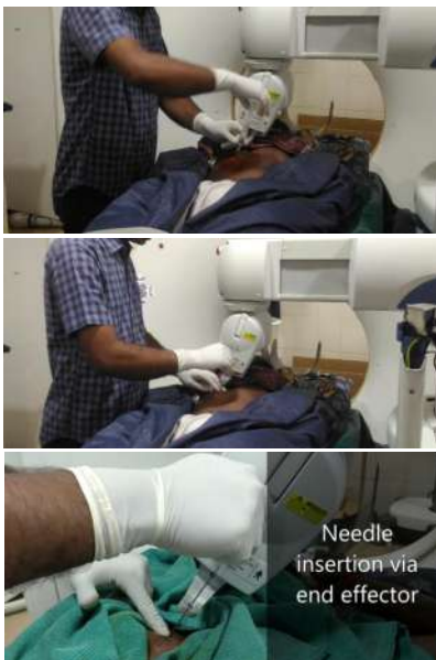
Fig. 4, 5&6: Robot-assisted Navigation system for CT-guided percutaneous lung procedures. Needle placement via the robotic arm at the location of planned pathway.
