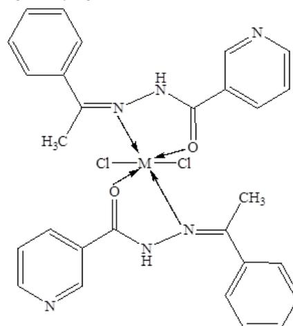
Figure 6: Proposed structure of metal complexes
