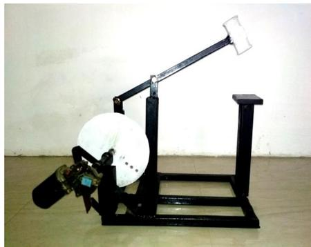
**Fig 3: Prototype Automatic Hammering Machine**
