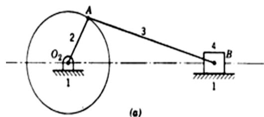
Fig 1: Slider Crank Mechanism
