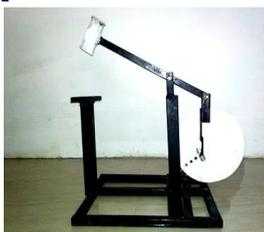
**Fig 2: Prototype Model Automatic Hammering Machine**
