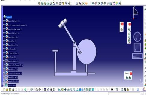
Fig 5: 3D View Of Automatic Hammering Machine
