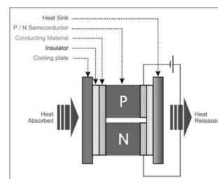
Fig 2.1: TEC construction
